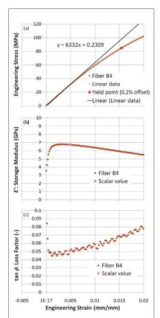
Figure 1. For one brown hair (B4), these are the simultaneous traces of (a) engineering stress, (b) storage modulus, and (c) loss factor, all as a function of engineering strain. The Young's modulus derived from the linear part of the stress-strain curve (a) is 6.33 GPa.
